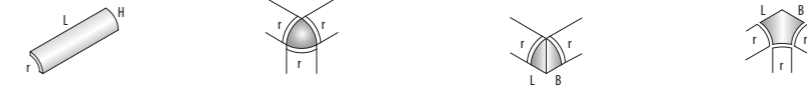
Radial tiles | 7,5 mm shaped pieces | radius 30 mm [average radius approx. 30 mm, ext. radius depending on the joint width up to 40 mm]
